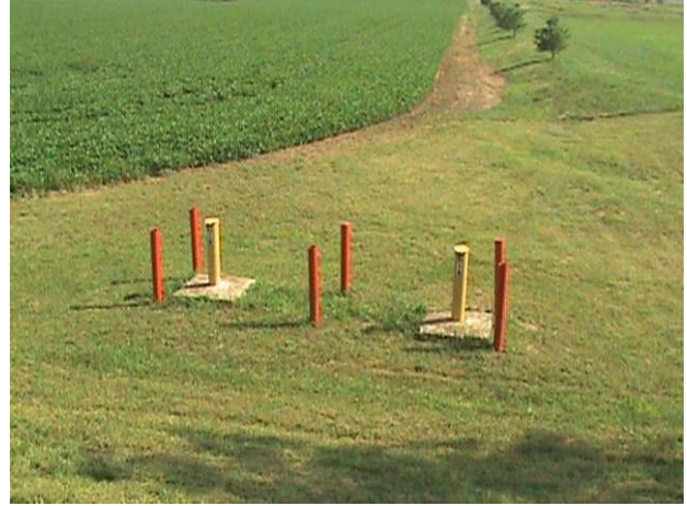
Monitoring wells in a non-commercial setting.
