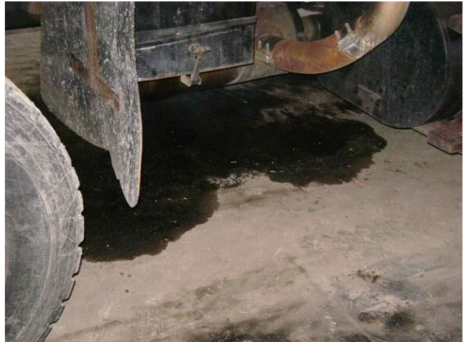
Surficial staining from a leaking vehicle. Presumably motor oil, but other possibilities include antifreeze, and transmission fluid.
