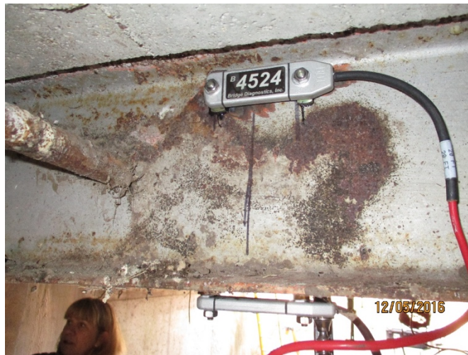
Fig. 48. Transducer attached to the top part of girder web at the same location as the bottom transducer
