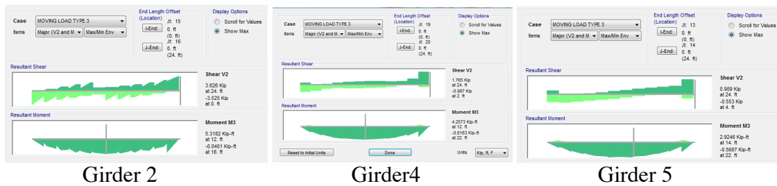
Fig. 10. Examples of moment and shear diagrams for mostly loaded girders (truck on lane 1 st )
