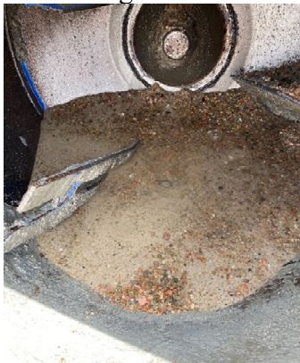
f) Clean aggregate covered with water
