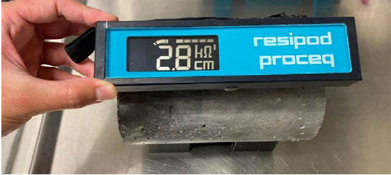
a) Surface resistivity measurement
