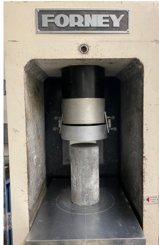
Figure 26. Compressive strength apparatus – Forney compression testing machine.
