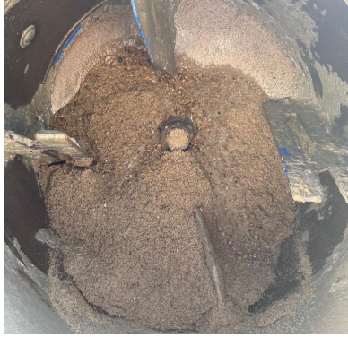
a) Loading of aggregate in the mixer
