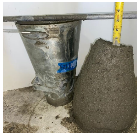
Figure 24. Slump test apparatus.
